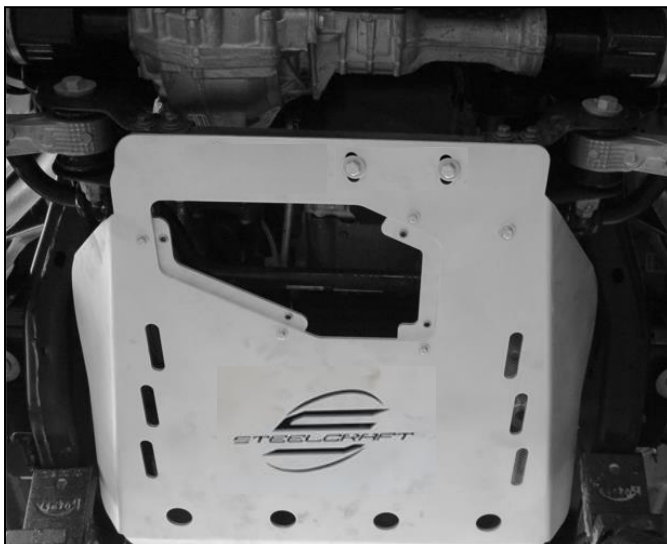
(Fig 14) Skid Plate attached to front crossmember
