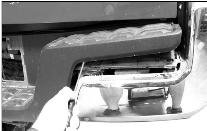
(Fig 10) Use a flat blade screwdriver to pry the plastic cover up from the top of the bumper to remove cover and access bumper mounting hardware
