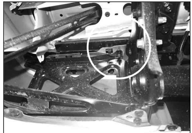
(Fig 9) Remove hardware attaching plastic top cover to top of receiver hitch (passenger/right side pictured from below/behind bumper)
