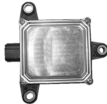
(Fig 17a) Disassemble factory bumper to remove Blind Spot Sensor (BSS) (MY18-21 pictured)
