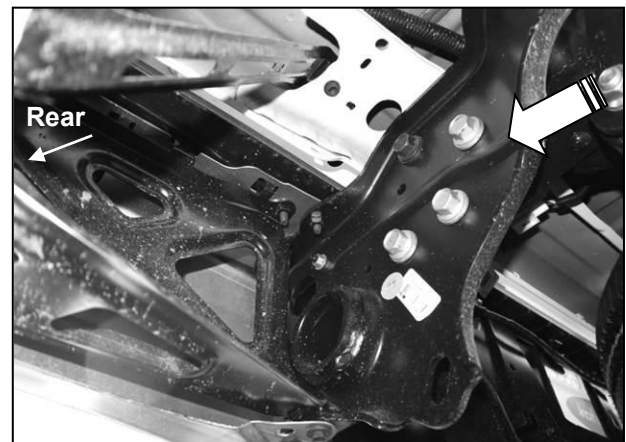
(Fig 2) Models without receiver hitch, remove hardware attaching bumper and brackets to side of frame to remove complete bumper assembly (passenger/right side pictured)
