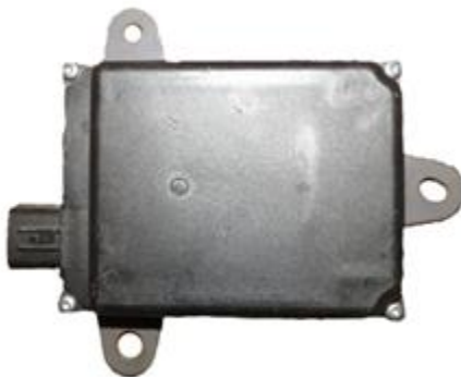
(Fig 17b) Disassemble factory bumper to remove Blind Spot Sensor (BSS) (MY14-17 pictured)
