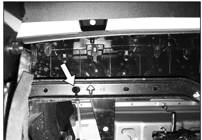
(Fig 8) Use a wire tie (arrow-not included) if needed to attach the bottom of the grille to the inner crossmember
