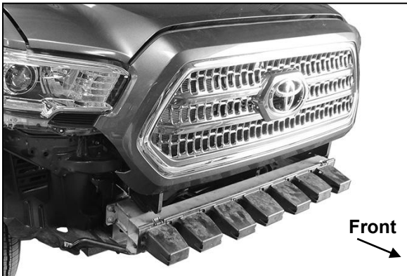
(Fig 5) Remove plastic impact bumper and aluminum crossbar from bumper brackets
