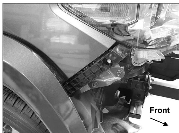
(Fig 4) Remove plastic block (arrow) from front edge of fender. Reinstall hardware to secure headlight
