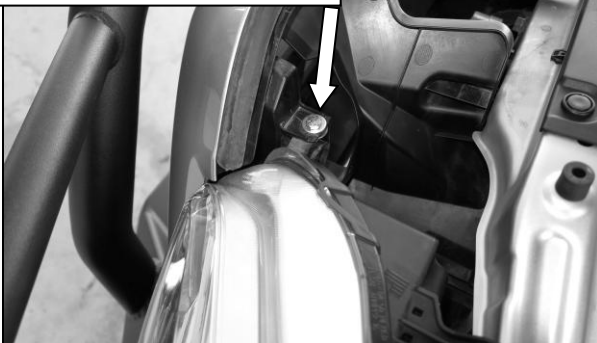
(Fig 7) Replace OE plastic pushpin with supplied hardware
