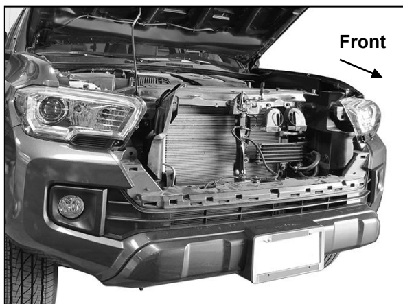
(Fig 3) Remove grille, air dam from below bumper and license plate. Remove plastic bumper cover
