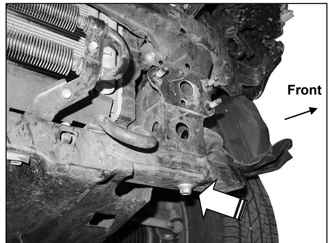
(Fig 6) Remove aluminum inner bumper from frame. Remove bolt (arrow) and set aside for reuse.
