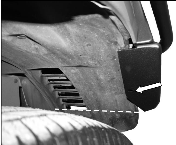
(Fig 23) Secure the fender liner to the bumper using the 6mm button head bolt through the mounting hole shown. Trim liner as necessary.
