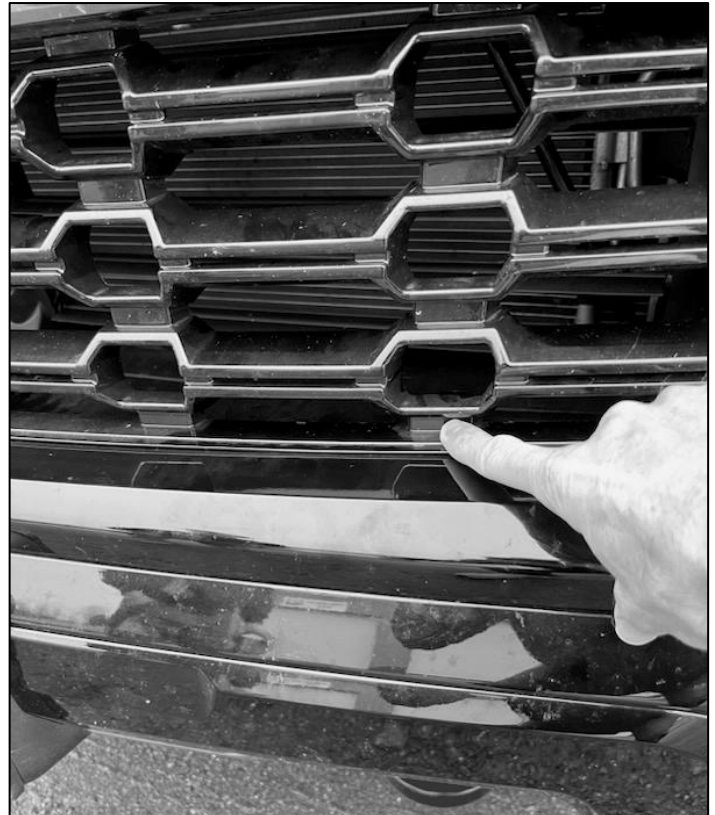
(Fig 15) Trim lower grille tab as needed to slide Top Support Bracket through the grille. (Tab example shown)
