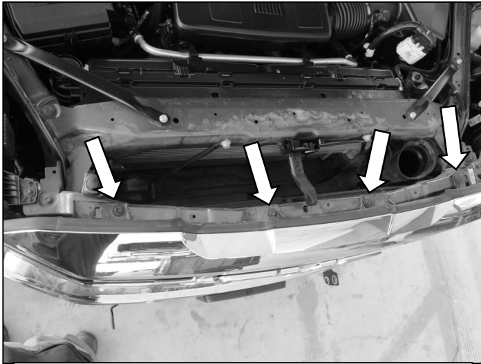
(Fig 13) Remove screws attaching grille (arrows)
