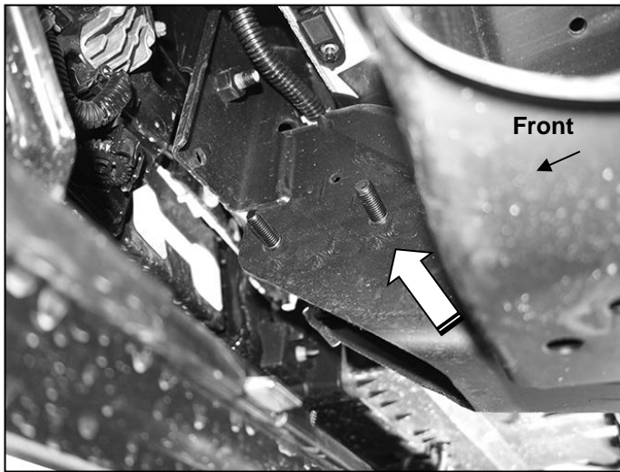
(Fig 10) Insert Double Bolt Plate through holes in outer side of frame
