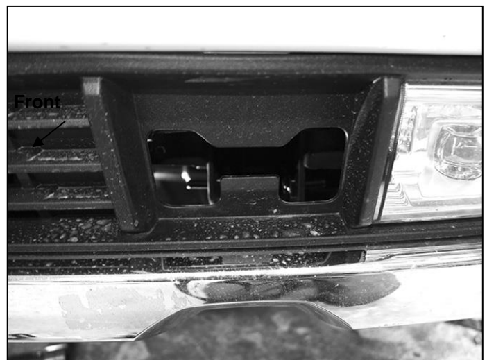
(Fig 9) Trim plastic opening if necessary, to clear Brackets
