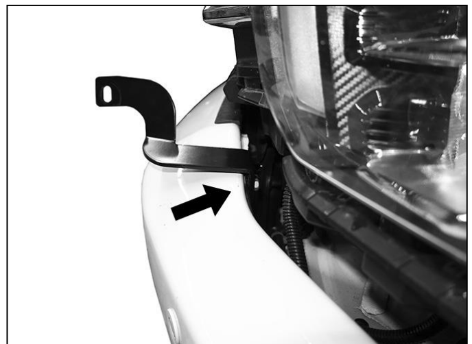
(Fig 5) From behind bumper, reuse bumper bolt to attach Driver/left Top Bracket to back of bumper bracket (arrow). Bumper pictured with top fascia body panel removed for instruction purposes only, do not remove fascia panel
