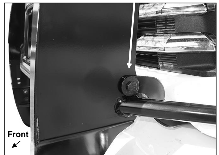
(Fig 17) Attach Top Bracket to outside of Grille Guard for 20-23 model years. (2024-on will mount inside)
