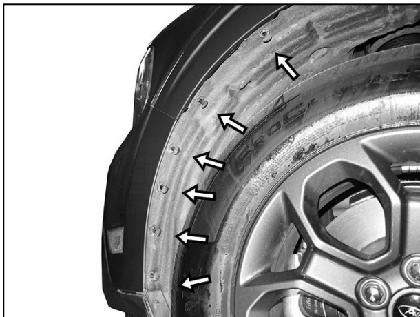
(Fig 3) Remove the screws/clips attaching the fender liner to the bumper and end of fender (driver/left side pictured)
