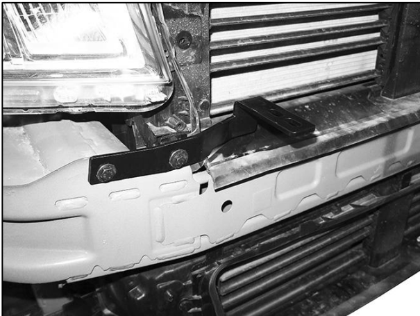
(Fig 14) Passenger/right Top Inner Support Bracket attached to crossbar
