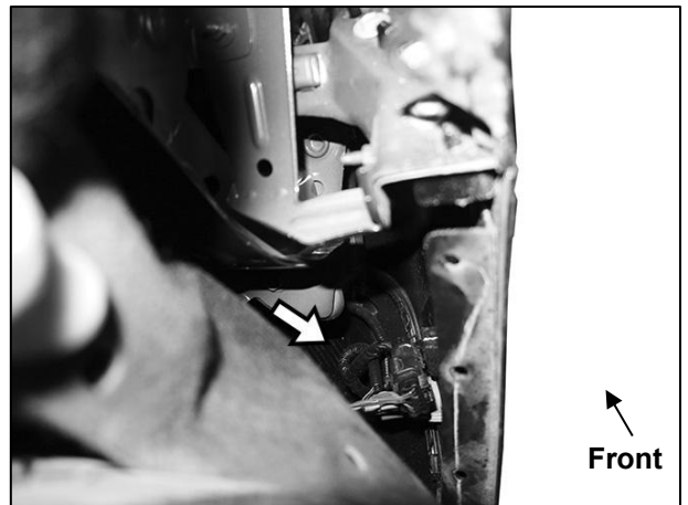
(Fig 8) Pull back liner and unplug the wiring harness leading to the front bumper (passenger/right side pictured). Remove hex bolts attaching bumper to fender (see Fig 5)
