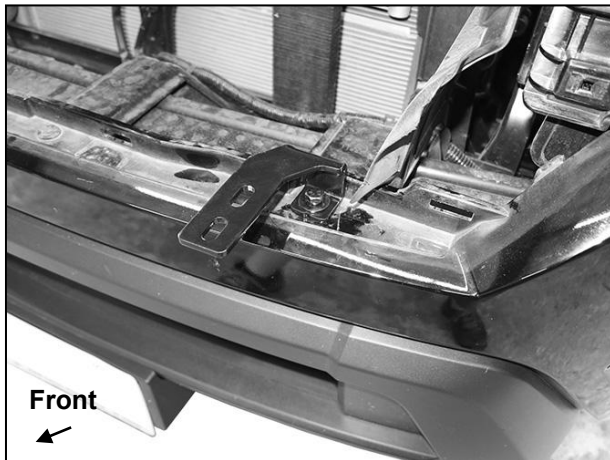
(Fig 13) Attach driver/left side Support Bracket to top of bumper
