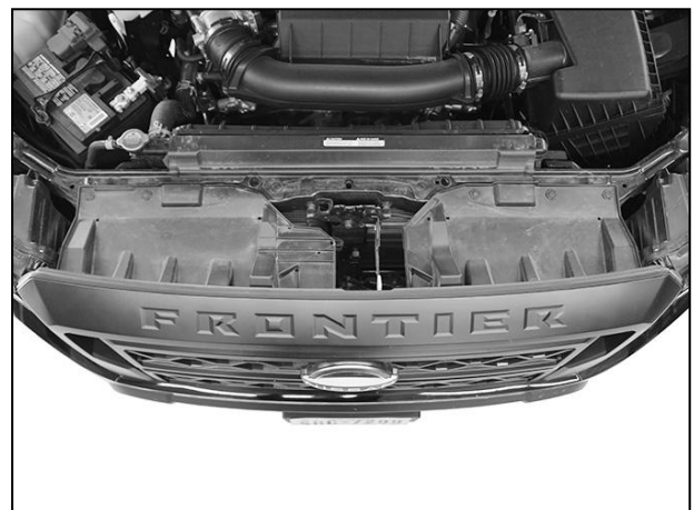
(Fig 9) Remove plastic cover and grille assembly
