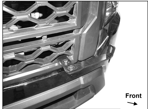
(Fig 17) Driver/left Guard Bracket installed
