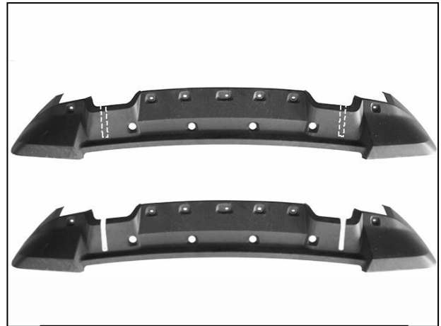
(Fig 21) Cut slots to clear the Brackets (dashed line for example only )
