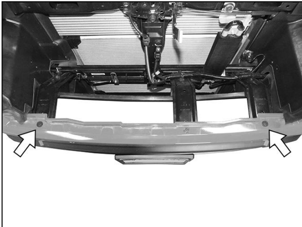
(Fig 11) Remove fasteners attaching top of bumper cover to steel bumper brackets (arrows)
