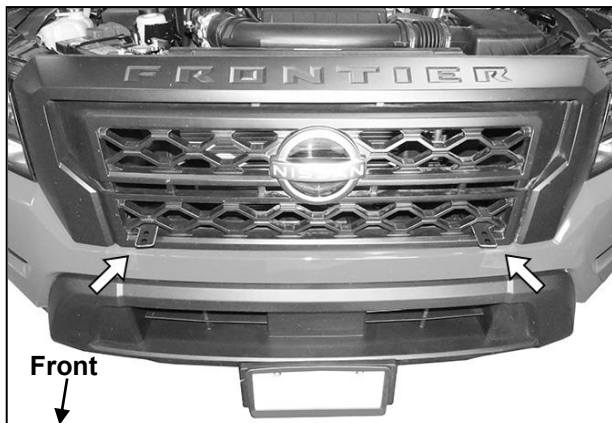
(Fig 15) Reinstall grille but leave loose. Guide Support Brackets through openings in grille (arrows)
