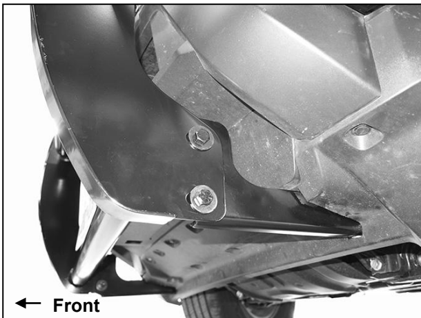
(Fig 22) Reinstall splash guard
