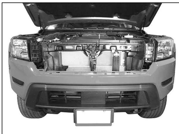
(Fig 10) Factory grille removed
