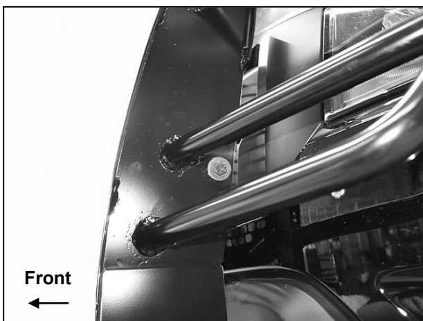
(Fig 20) Attach driver/left Guard Bracket to inside of Grille Guard upright
