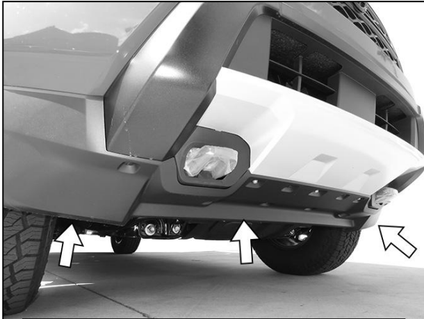
(Fig 1) Model with splash guard (arrows)
