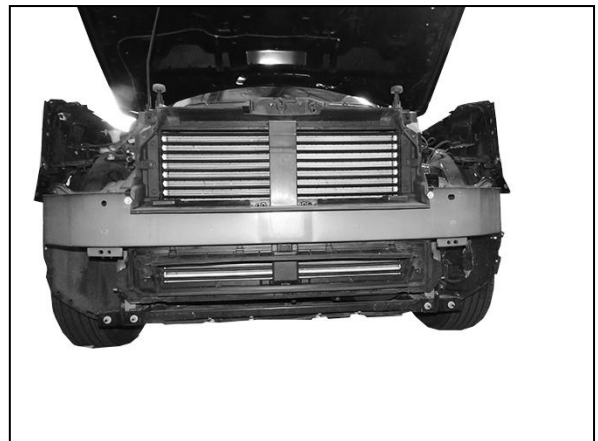
(Fig 10) Carefully remove the bumper cover assembly and place it on a clean, soft surface
