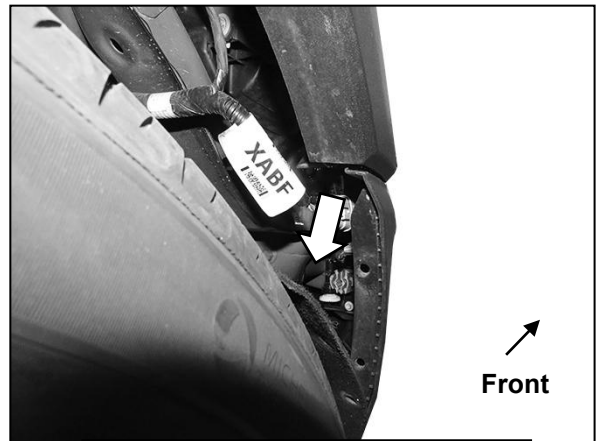
(Fig 6) Unplug the wiring harness leading to the front bumper (passenger/right side pictured).
