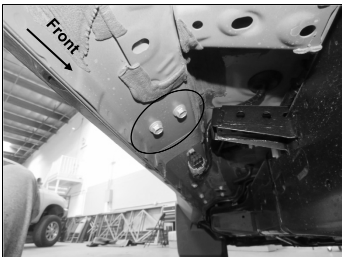
(Fig 4) Locate the center mounting points circled and remove the OEM 8mm bolts.
