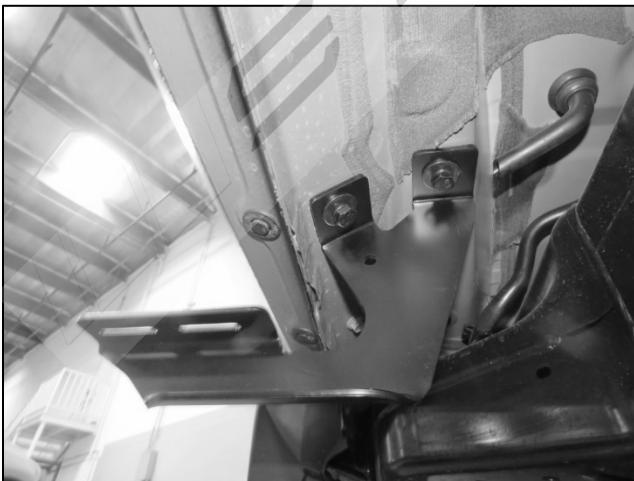
(Fig 3) The Front Mounting Bracket is installed.
