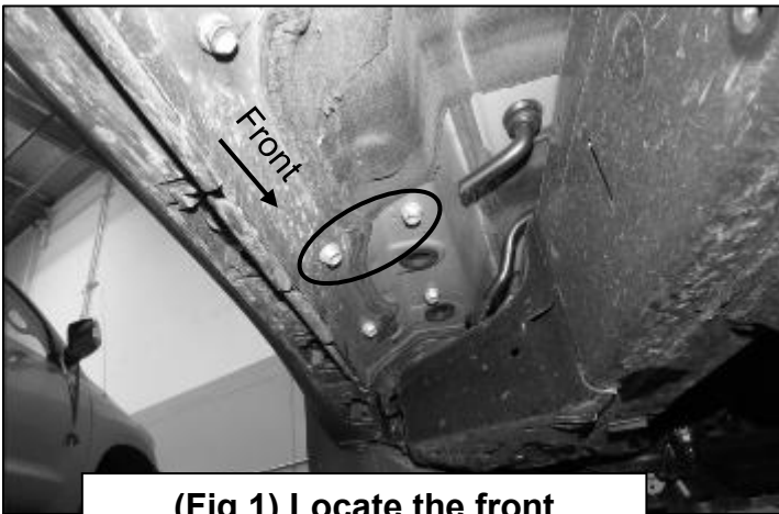
(Fig 1) Locate the front mounting location circled and remove the OEM 8mm bolts.
