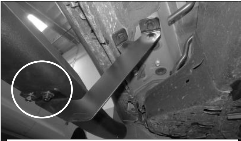
(Fig 7) Ensure the side bar sits flush onto the mounting brackets. Make adjustments if needed.
