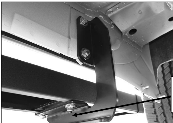
(Fig 10) Driver/left front mounting Bracket installed
