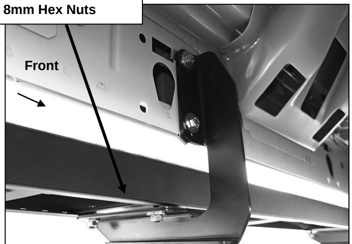
(Fig 11) Driver/left center Mounting Bracket installed
