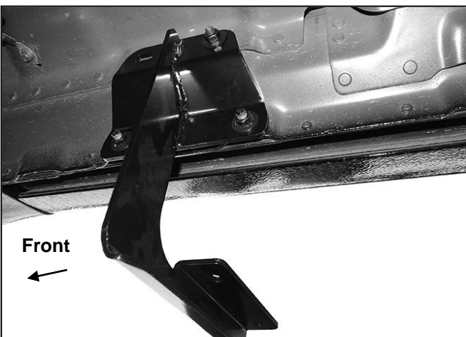
(Fig 5) Passenger/right front Bracket installed
