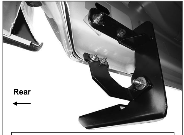
(Fig 17 Driver/Left rear Brackets installed)
