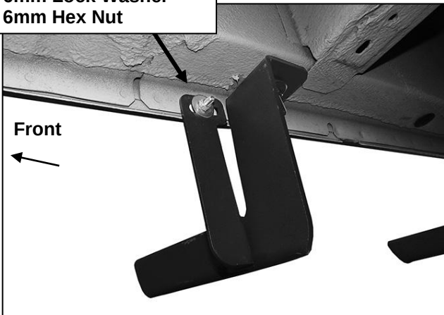
(Fig 18) Passenger/right center Brackets installed
