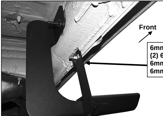
(Fig 11) Mark and drill hole through pinch weld. Attach top of Driver/left front Support Bracket to back of pinch weld. Reinstall Running Board
