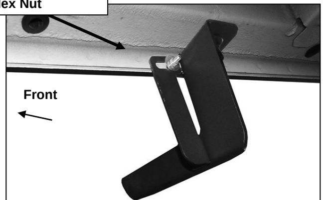
(Fig 19) Passenger/right rear Brackets installed
