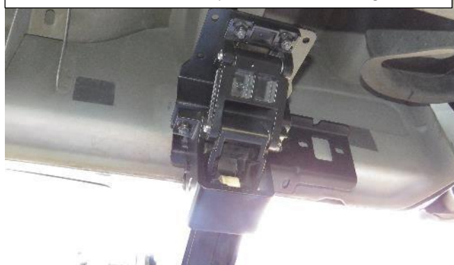
Rear bracket assembly mounted to Mega Cab
