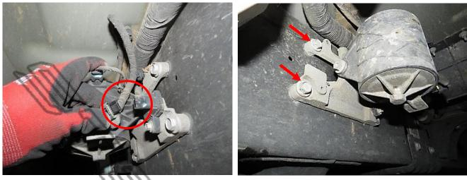
Locate Relcation Bracket (Left) (P) and M8 Carriage bolts. Insert M8 Carriage bolts (O) through the square holes on the Relcation Bracket (P) and secure using Plastic Insulators (F). This will keep the carriage bolts from falling out of the holes on the bracket.
