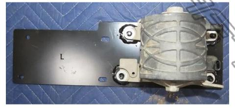
Mount the Relocation Bracket (P) onto the vehicle's Driver Side frame where the ATMM was using the OE flanged bolts. Be sure to fasten all hardware fully.
