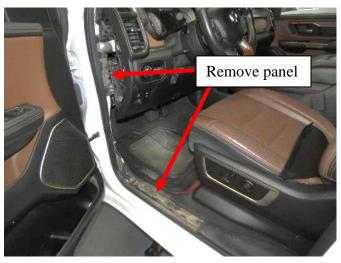
Locate the green CAN wiring hub on the backside of the metal framework. Carefully remove the entire black plastic casing (with the green wiring hub attached) by pulling it up. On some models a plastic detent may need to be pressed to unhook the plastic casing from the metal bracket. Carefully pull the plastic hub out of the side cavity for ease of reach.
