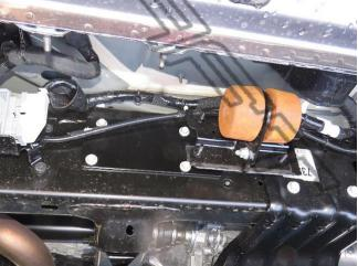
On some vehicles like the TRX, an OE module plug may be in the way. If so, unbolt the plug's bracket from the frame. Then remove the plug from the bracket. Plug may be located at the front or rear.
