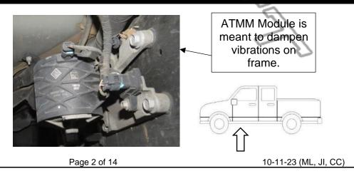
Locate Driver Side ATMM module on frame. Unplug ATMM module. Remove ATMM module from frame by unbolting fasteners.
