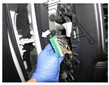
Identify the configuration of the plugs on the CAN Bus hub. On the row with empty slots, select the closest plug with two wires extending from it. The wire closer to the center of the hub is the CAN High wire. The wire further towards the outer edges is the CAN Low wire.
