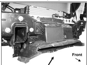
(Fig 34) 2022-on model tow hook reinstallation. Models with intercooler (turbo gas or diesel engines) must unplug and remove shroud and shutter assembly
