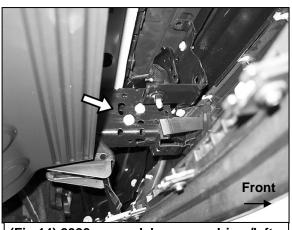
(Fig 14) 2022-on model, remove driver/left tow hook (pictured from behind bumper)
