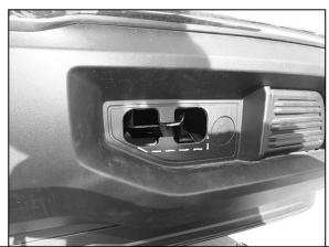
(Fig 3) Tow hook removed. Opening may need to be trimmed to clear the Mounting Bracket
