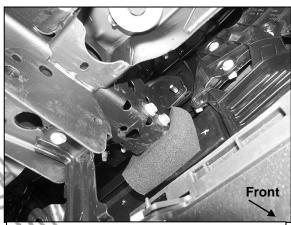
(Fig 2) 2019-21 model passenger/right tow hook pictured from behind bumper
