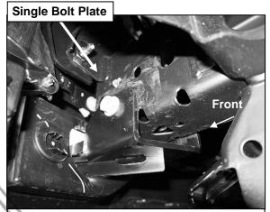
(Fig 6) Attach Driver/left Mounting Bracket assembly to end of frame with Bolt Plates
