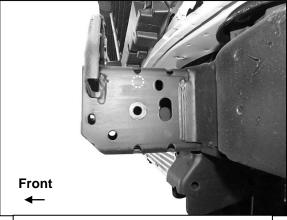
(Fig 36) 2022-on model tow hook reinstallation, use a 1/2" drill bit to drill a new mounting hole. Driver/left outer side of frame pictured
