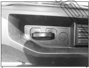
(Fig 1) 2019-21 model driver/left tow hook
