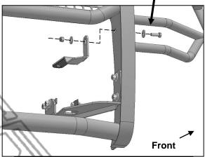
(Fig 42) Attach Grille Guard to 2022-on model driver/left side Top Bracket
