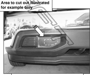
(Fig 4) 2019-21 passenger/right side model without tow hooks. Dashed line for example of cut only
