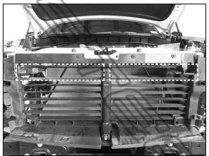
(Fig 25) 2022-on model, remove the upper blades from the shutter assembly
