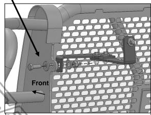
(Fig 45) On 2022-on models, attach Outer Top Bracket to Grille Guard. Driver/left side Brackets illustrated
