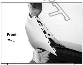
(Fig 18) 2022-on model, remove plastic body panel between headlight and bumper, (fascia)
