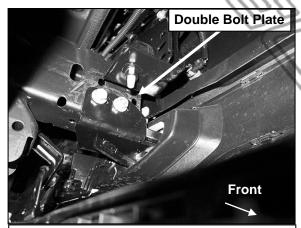
(Fig 7) Attach Driver/left Mounting Bracket assembly to end of frame with Bolt Plates
