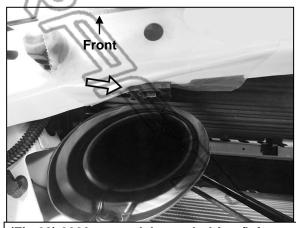
(Fig 28) 2022-on model, attach driver/left Inner Top Bracket to back of core support
