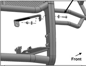
(Fig 41) Attach Grille Guard to 2019-21 model driver/left side Top Bracket
