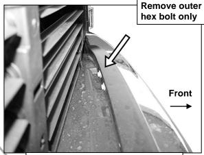
(Fig 11) 2019-21 Model, driver/left side top mounting location
