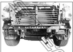
(Fig 35) 2022-on model tow hook reinstallation. Remove bumper, outer shroud and inner shutter assembly
