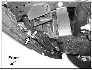
(Fig 32) 2022-on model tow hook reinstallation, remove hardware attaching bottom of bumper to driver/left side bracket (arrow)
