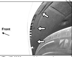
(Fig 17) 2022-on model, remove the hardware attaching fender liners to fenders
