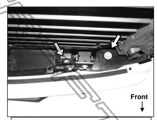
(Fig 33) 2022-on model tow hook reinstallation, remove hex bolts attaching bumper bracket and remove bumper
