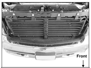
(Fig 9) Remove screws attaching grille and carefully pull grille straight out to remove
