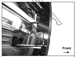
(Fig 43) Attach Grille Guard to driver/left side Brackets. 2022-on model pictured
