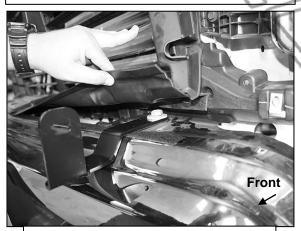
(Fig 22) 2022-on model, reuse hex bolt to attach driver/left Support Bracket to top of bumper bracket
