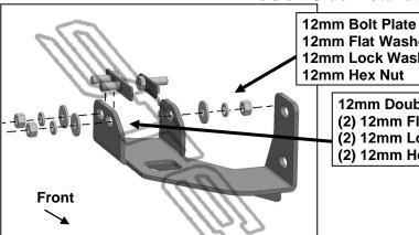
(Fig 5) Attach Driver/left Mounting Bracket to end of frame with Bolt Plates
