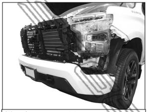
(Fig 20) 2022-on model, remove fascia body panel from top of bumper and remove grille
