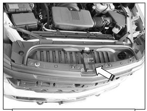
(Fig 19) 2022-on model remove hood release lever and cover, (arrow). Also remove grille
