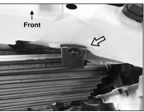
(Fig 29) 2022-on model, attach passenger/right Inner Top Bracket to back of core support
