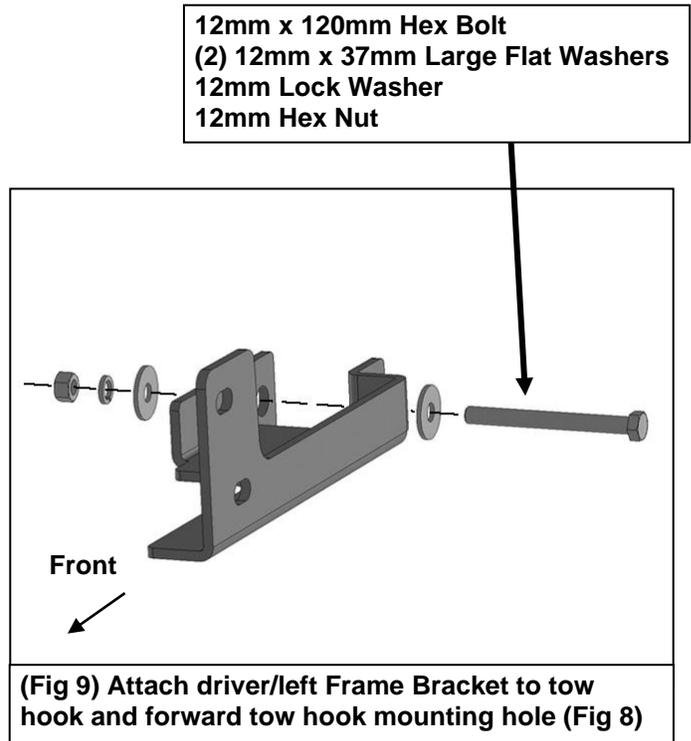
Driver/left Frame Bracket to tow hook and forward tow hook mounting hole
