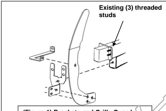
**(Figure 1) Brackets and Grille Guard Mounting Locations**
