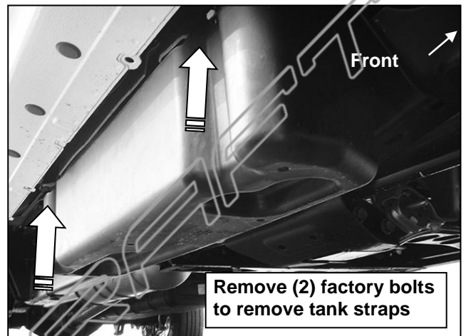
(Fig 12) Passenger side DEF tank and cover Remove (2) factory bolts to remove tank straps
