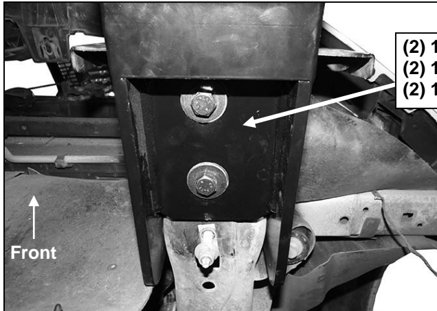
(Fig 6) Driver/left Frame Bracket pictured from below
