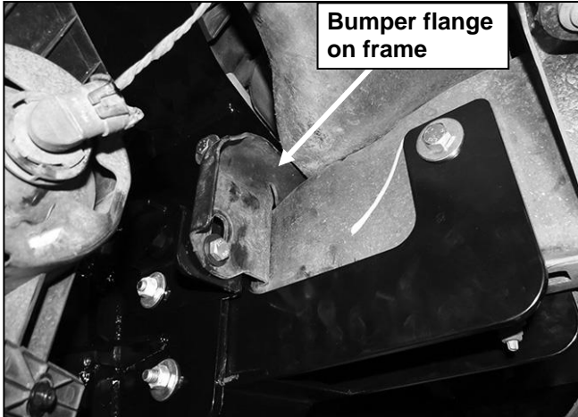
(Fig 15) Attach Outer Support Bracket to flange on frame and center hole in Bumper Bracket
