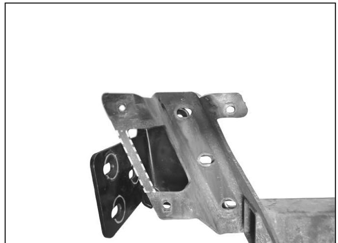
(Fig 6) On year models 06-08 with factory receiver hitch, trimming is required on factory bumper support in order to re-use tow hitch
