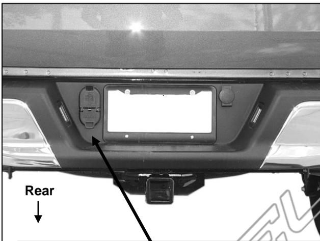
**(Fig 1) Unplug and remove 7-wire trailer plug**
