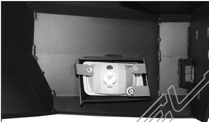
**(Fig 16) Remove (3) screws from lights. Adjust tabs on Bumper if necessary to line up with light. Reuse screws to attach light to tabs on Bumper.**
