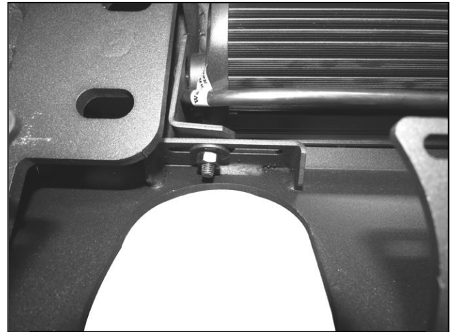
(Fig 21) Light bar attached to LED Brackets pictured from the back of the bumper
