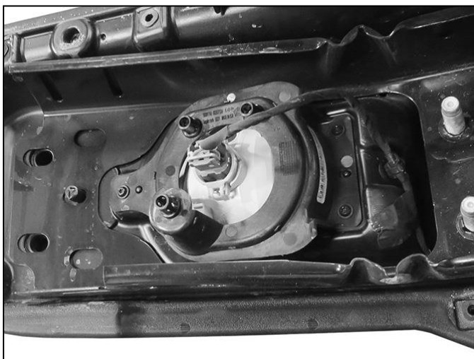
(Fig 14) 2018-on Sport model with 1pc plastic bumper cover. Driver/left Fog light assembly pictured
