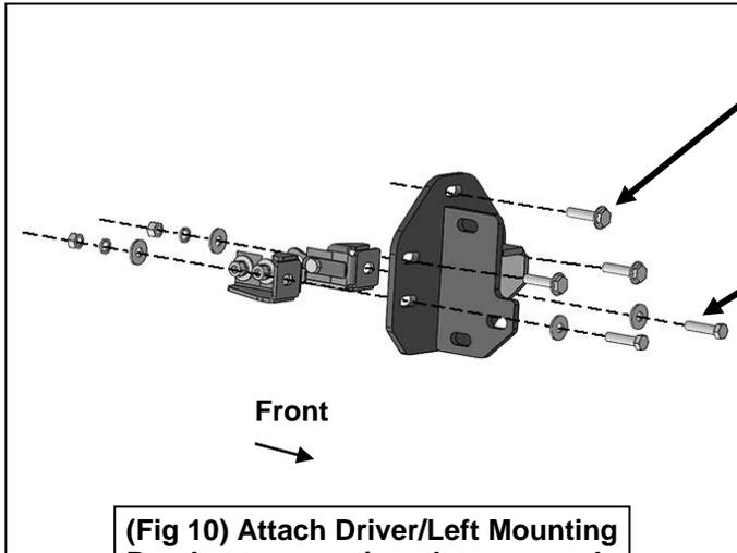
Reuse (3) factory bumper bolts to attach Bracket to factory frame bracket
