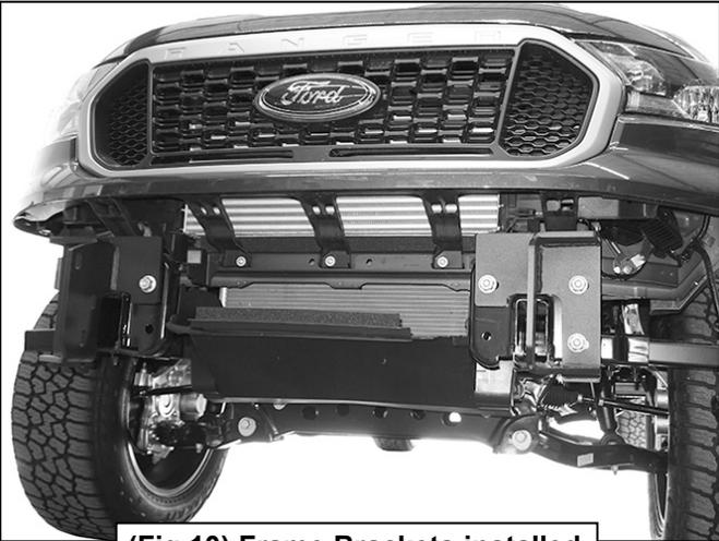
(Fig 10) Frame Brackets installed
