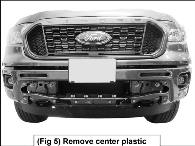
(Fig 5) Remove center plastic bumper cover and license plate
