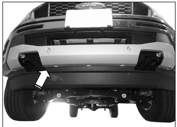
**(Fig 4) Remove the center plastic cover**
