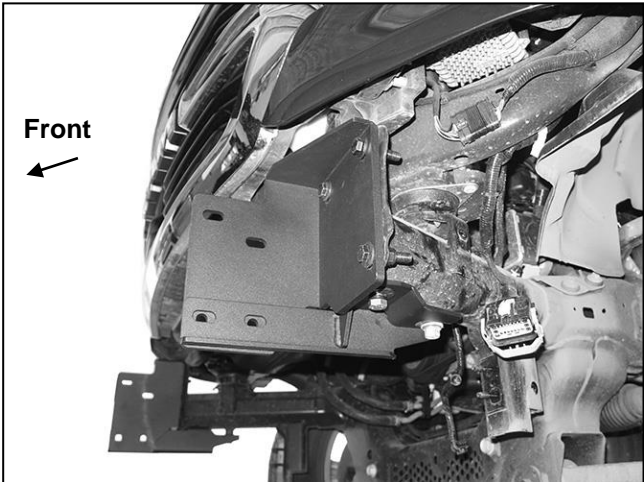
(Fig 7) Frame and Support Brackets installed
