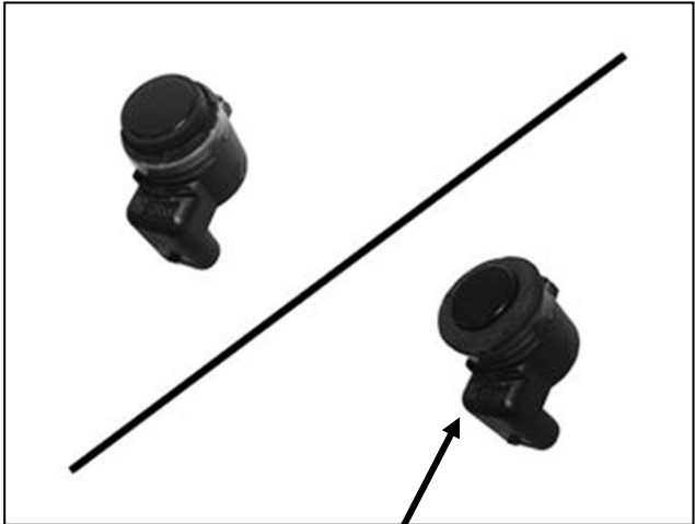
(Fig 10) Remove silicone seal from sensor. Slide large Seal over end of sensor (arrow)
