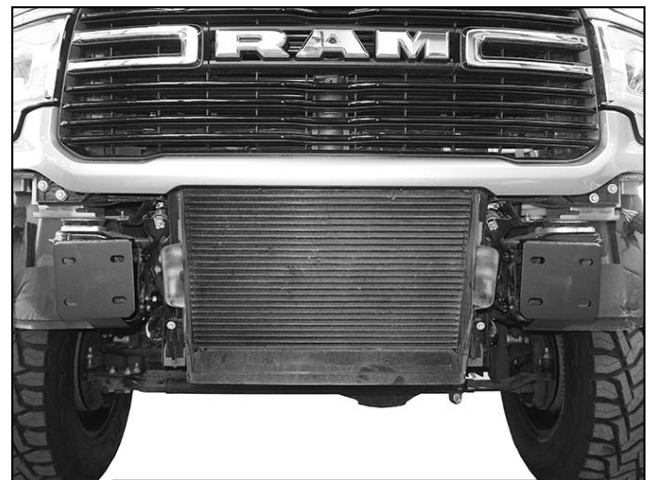
(Fig 4) Frame Brackets installed
