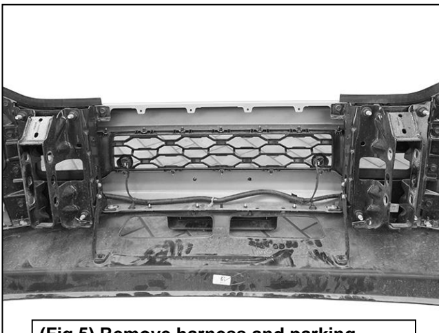
(Fig 5) Remove harness and parking sensors from factory bumper if equipped
