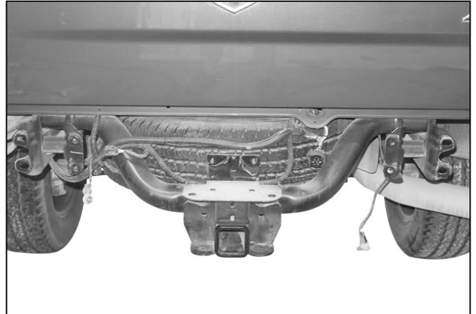
**(Fig 8) Example of factory bumper bracket with 8mm hex nuts (inner) welded onto back of bumper bracket**
