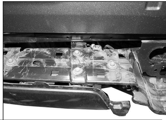
**(Fig 4) Models with receiver hitch, remove the hex bolts attaching top of bumper**
