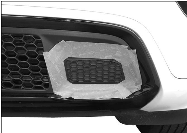
(Fig 11) For models with one piece bumpers, cutting is necessary. Mark the location with tape. Cut the grille to access the mounting location
