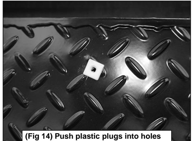
**(Fig 14) Push plastic plugs into holes in Bumper for license plate if required**
