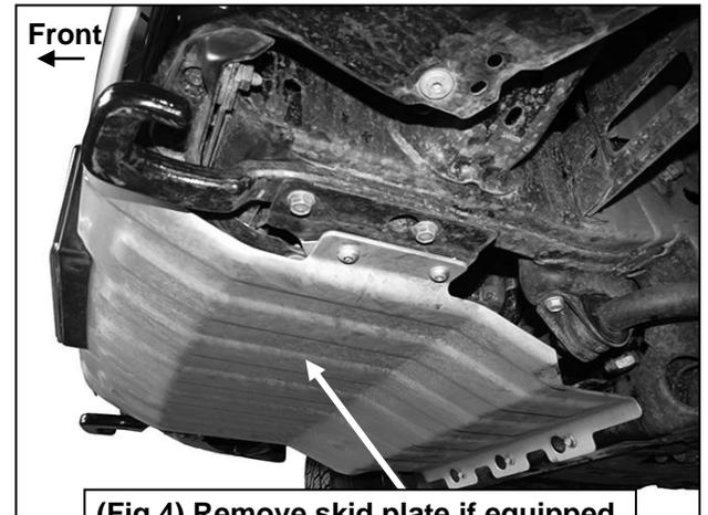
(Fig 4) Remove skid plate if equipped
