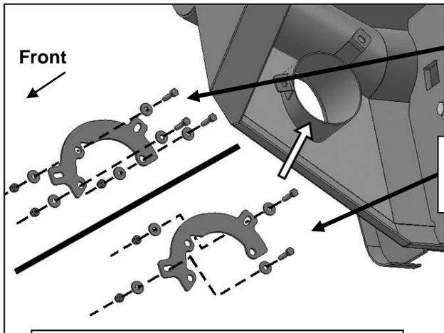
Attach the Adapter Bracket to the fog light first if equipped
