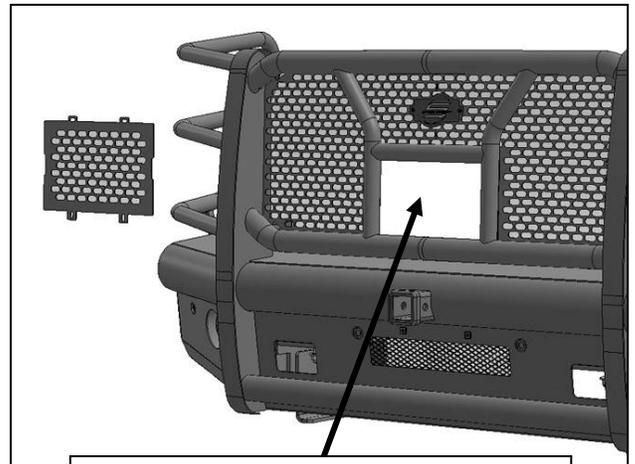
(Fig 18) Remove screen from grille for models with grille mounted camera
