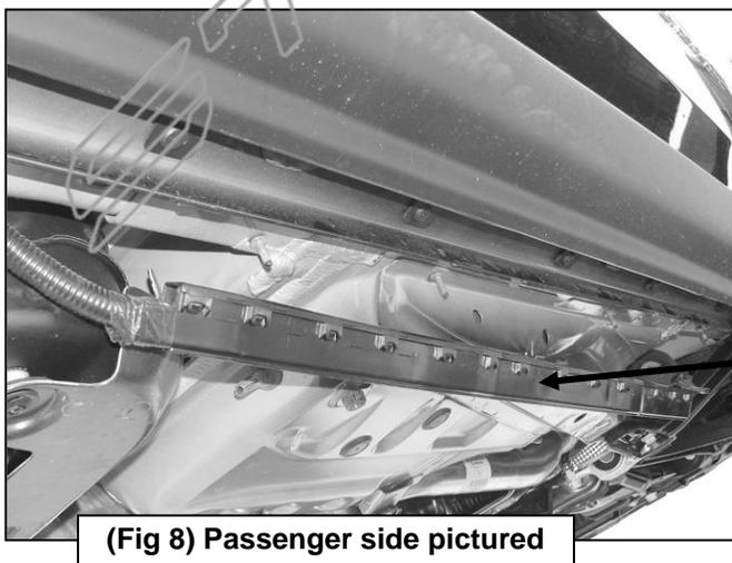
Remove hex nuts from wiring harness.
