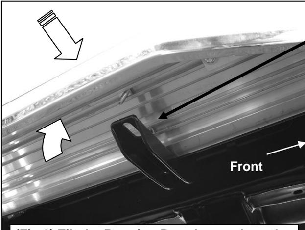
Slide T-Bolt along slots to line up with Mounting Brackets
