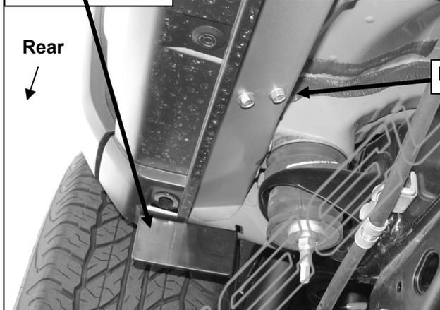
(Fig 3) Passenger side rear bracket location pictured
