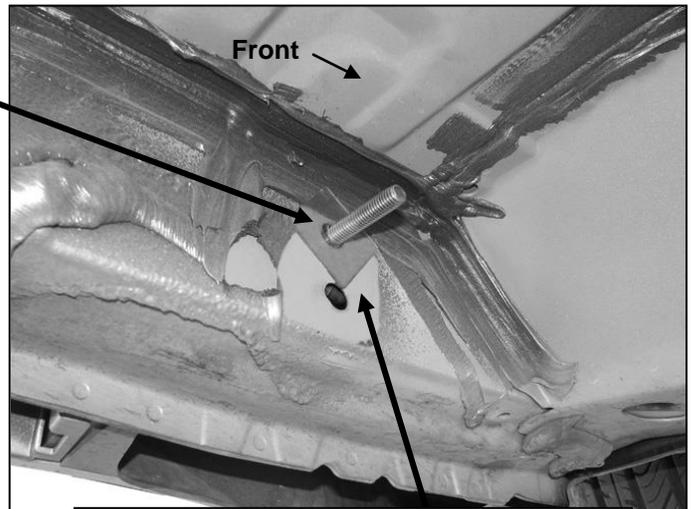
(Fig 3B) Use Plastic Retainer to hold Rod
