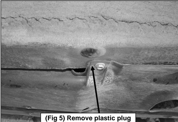
(Fig 5) Remove plastic plug on bottom of frame channel
