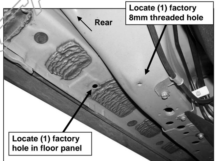
(Fig 9) Driver side rear mounting location pictured
