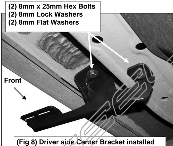
(Fig 8) Driver side Center Bracket installed
