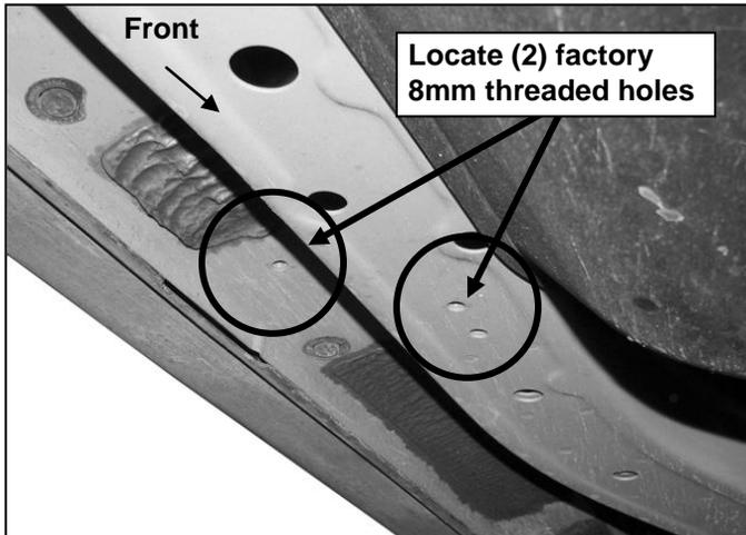
(Fig 6) Driver side center mounting location pictured
