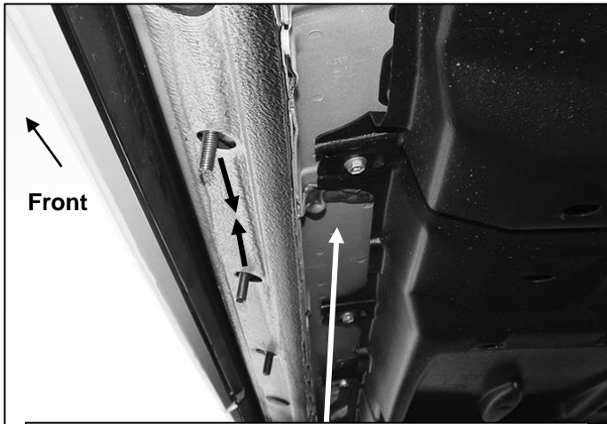
Fig 3) Scrape excess body sealant as necessary from all locations before installing Brackets
