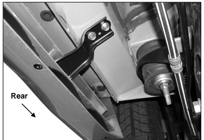
**(Fig 4) Passenger side rear bracket location pictured**
