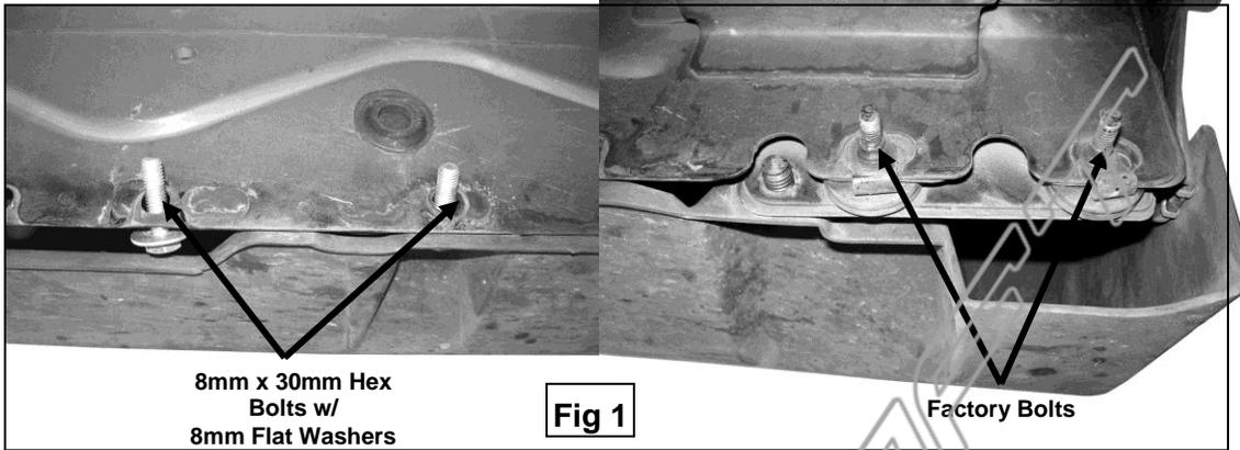
Pinch Weld Rear Mounting Location
