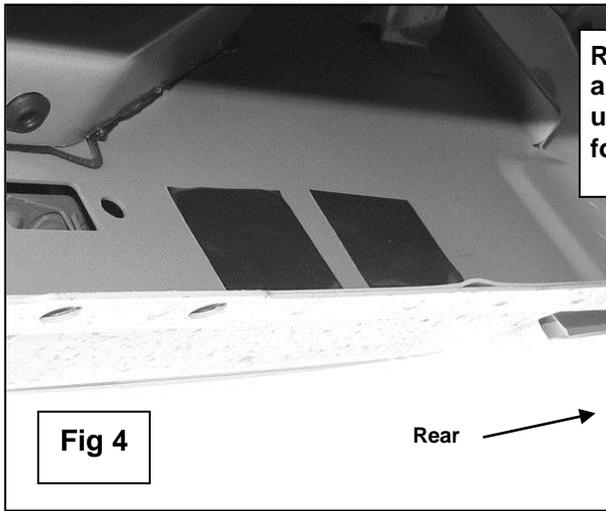
Remove sealing tape and/or rubber grommets to uncover the rear location for the Mounting Brackets
