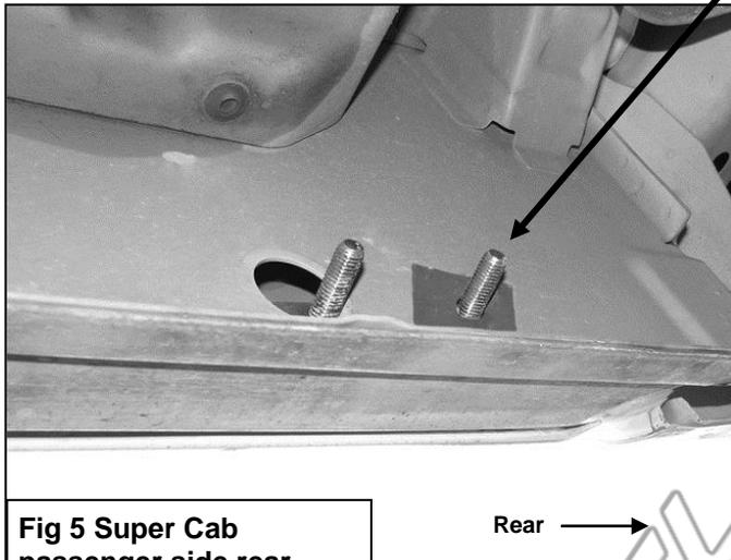
Fig 5 Super Cab passenger side rear mounting location pictured. Shown with Plastic Retainer in place
