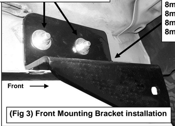
**(Fig 3) Front Mounting Bracket installation**
