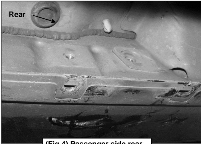
**(Fig 4) Passenger side rear mounting location pictured**
