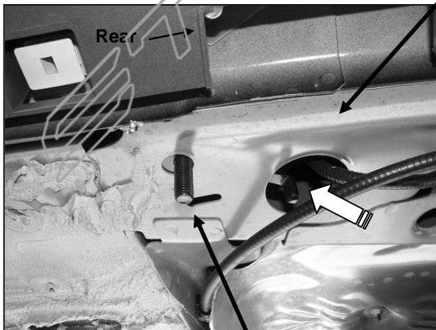
(Fig 19) Insert 12mm Bolt Plate into large hole and out smaller hole
