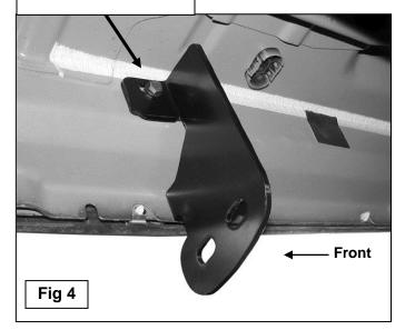
10mm x 25mm Hex Bolt (2) 10mm Flat Washers 10mm Nylon Lock Nut
