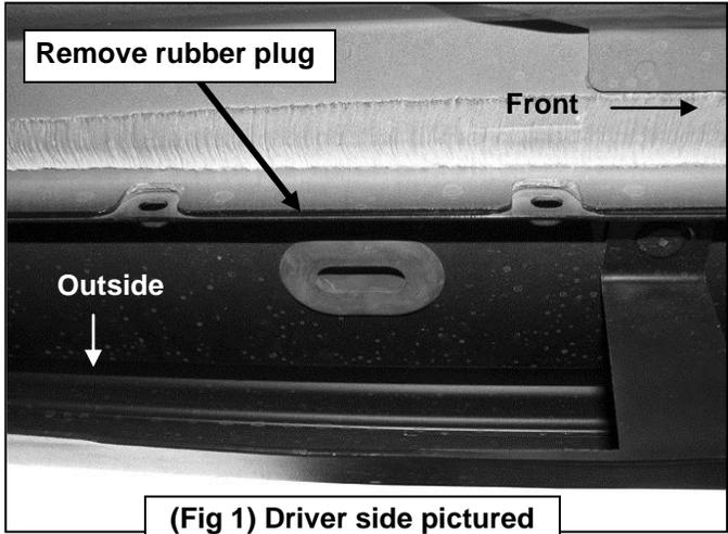
(Fig 1) Driver side pictured from below vehicle
