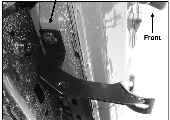
(Fig 4) Driver/left front Mounting Bracket installed
